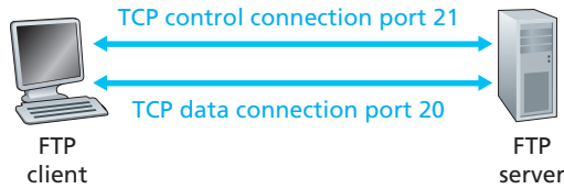
Figure 2.15 ♦ Control and data connections
